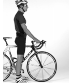
Figure 1- Minimum stand-over height A = 1" (25 mm) for most bicycles 2-3" (50-75 mm) for mountain bicycles
