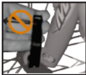
Figure 40- Test for rotation
