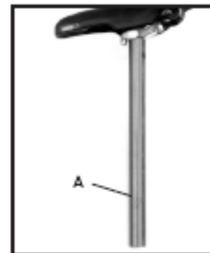
Figure 19- Minimum insertion mark on seatpost A- This line must be inside the bike frame
