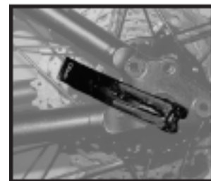
Figure 37- Rear lever position
