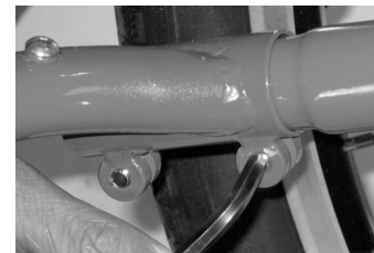
Fig 3: Tighten sideloader sleeve
